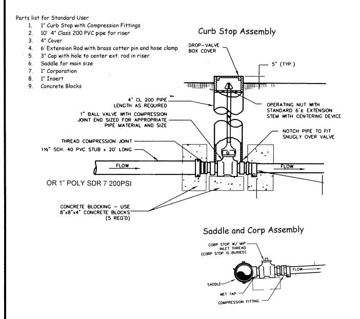
GRWD will provide each member a curb stop assembly, properly sized saddle and 1'' corp. GRWD will perform a wet tap on the main.
